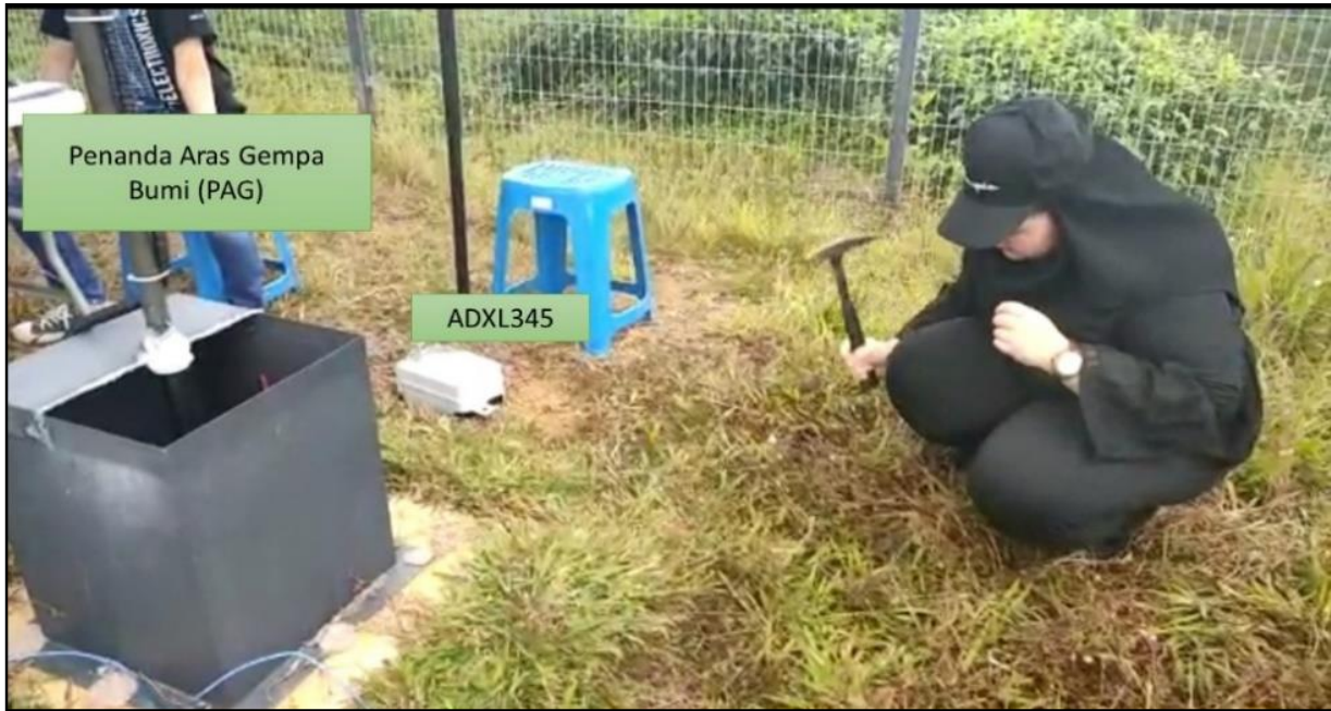
Figure 2: Placement of PAG and ADXL345 is in distance 1.0m and force is given from 3.0m away of both devices.
