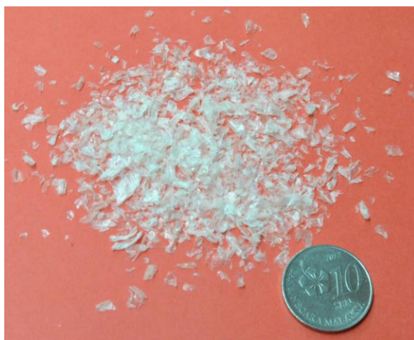
Figure 2. The physical appearance of chitosan produced by using shrimp shell as raw material.
