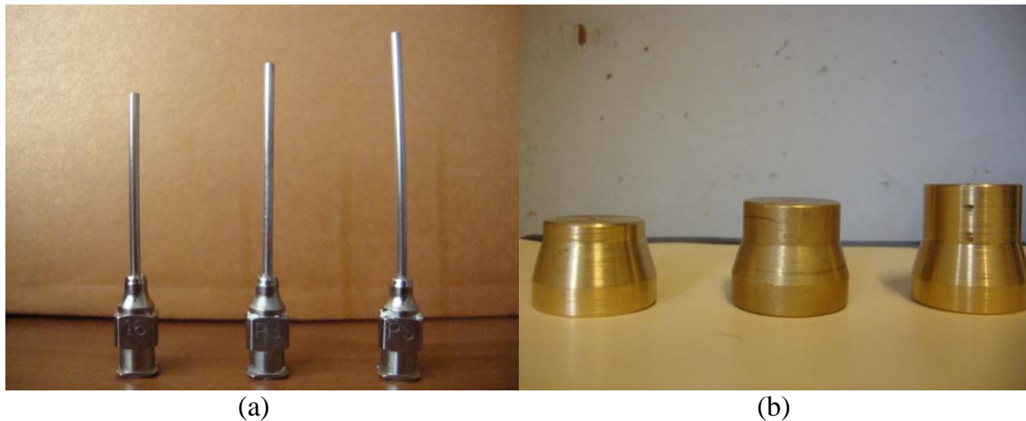
Figure 3. (a) Nozzle Length in 29 mm, 34 mm, and 39 mm; (b) Cap Nozzle
