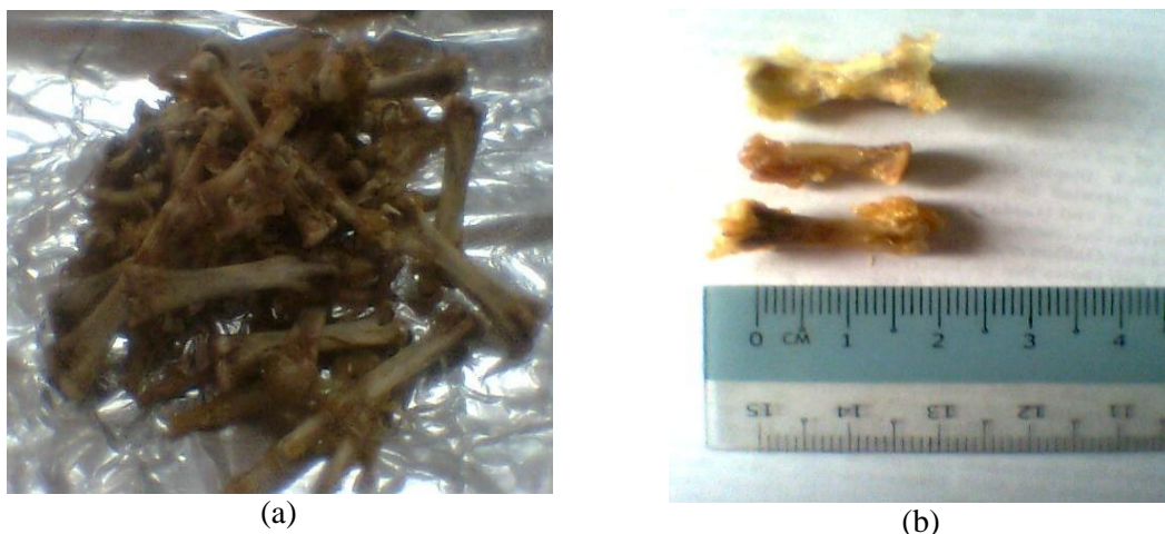
Figure 1. Chicken feet bones obtained for gelatin extractions (a) Dried samples at 50°C for 18 hours; (b) Bones cut to small size, 1 – 3 cm.
