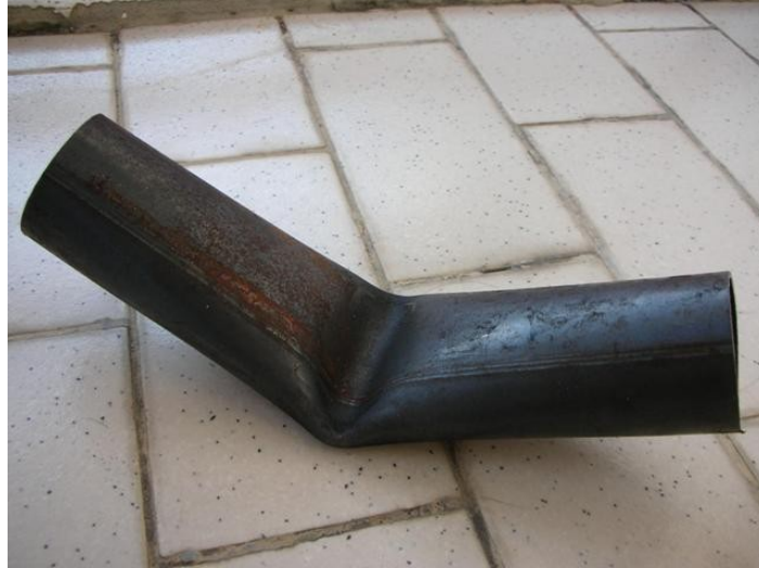
Figure 7. Deformation of thin wall tube after three point bending test
