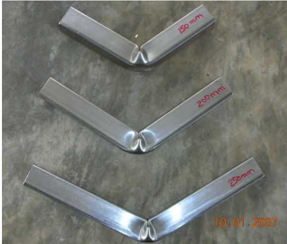
Figure 6. The deformation shapes of the specimens after three points bending test
