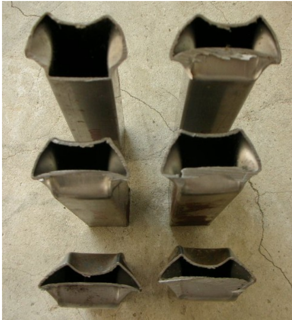
Figure 7. Cross sectional at the deformed area of thin walled tubes
